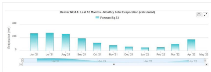
A user-friendly dashboard that calculates theoretical total evaporation using publicly available NOAA meteorological data.
