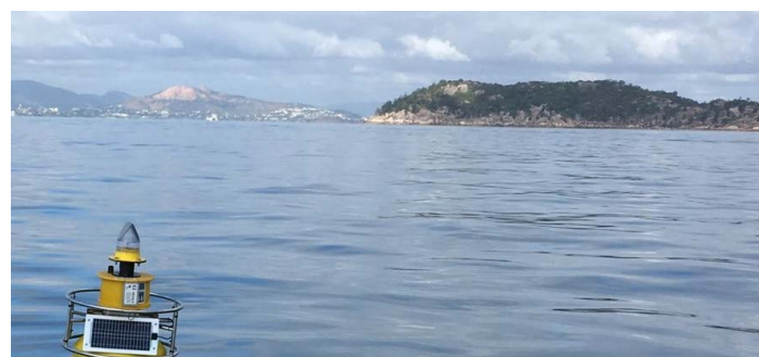
POTL Marine buoy with Xylem EXO and Gill Water Quality Sensors.
