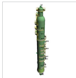
Vertical pressure vessel with platforms and staircase.
