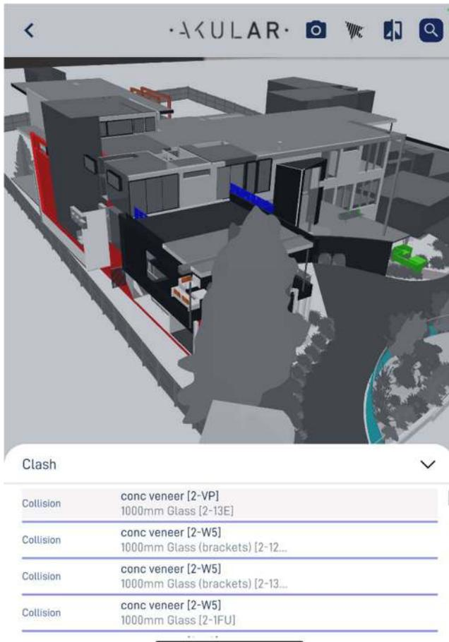
Caption: The powered by iTwin platform helps Akular users detect collisions and check the clearance between geometric elements.
