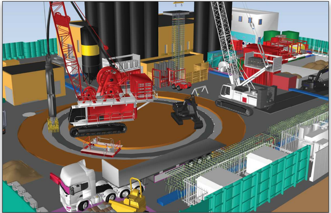
Using SYNCHRO 4D, CVB JV created over 30 4D models to analyze constructability and streamline construction planning.
